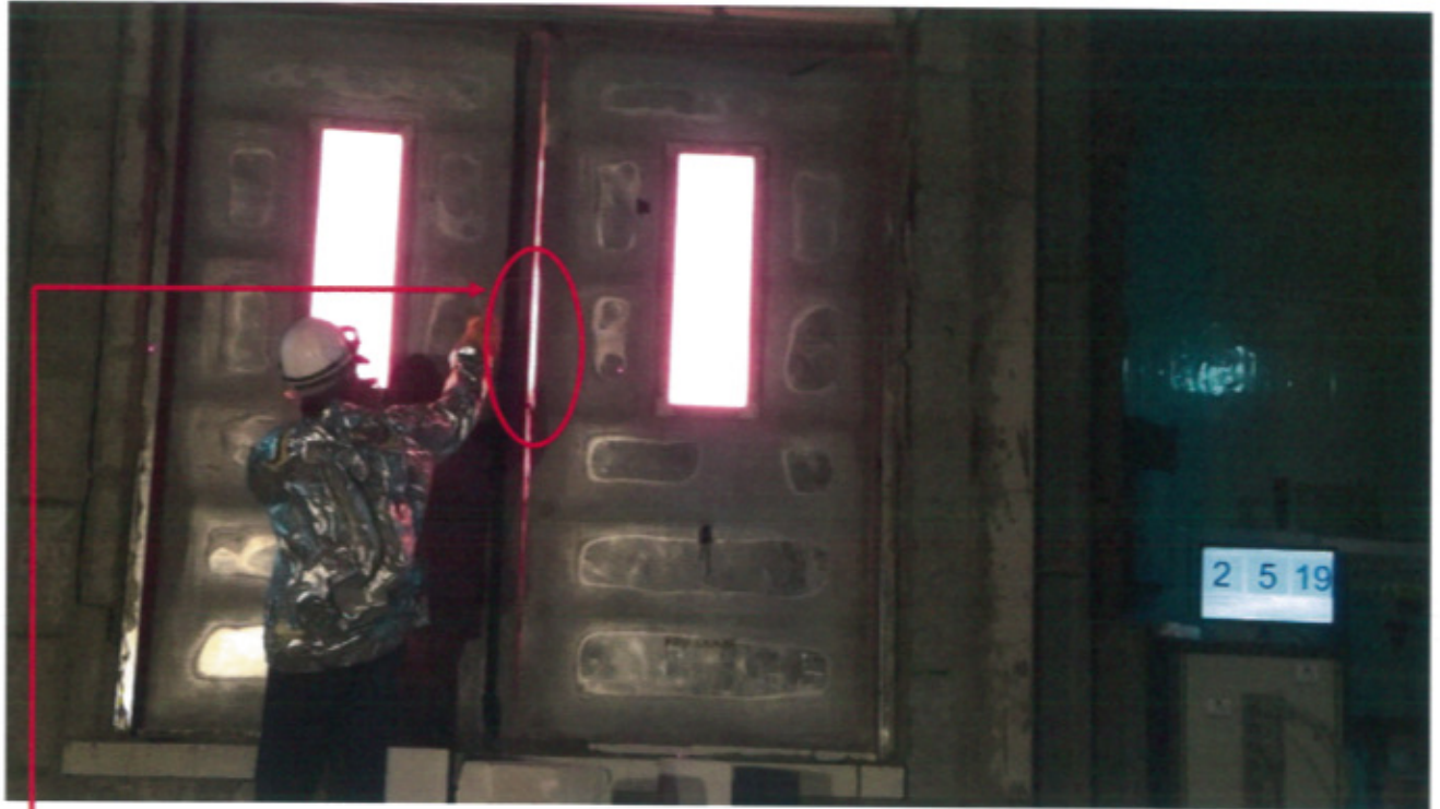
Penetration of and 150mm vertical movement of 6mm gap gauge at mid-height of meeting stile after 125mins of testing
